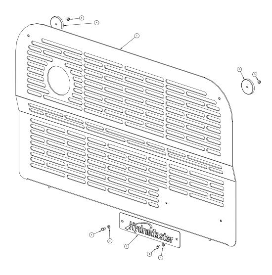
Figure 1-33 Machine Left Side Cover Assembly D-5587 Rev -
