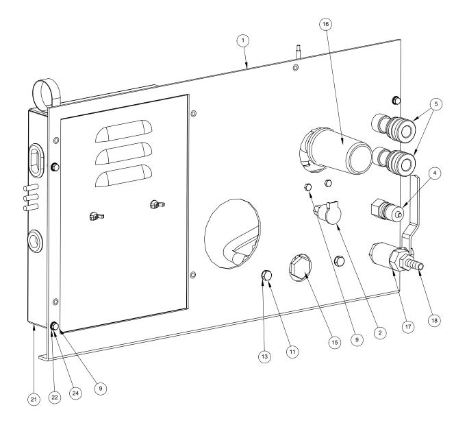
Figure 1-25 **Dash Lower Assembly - Rear View** D-5577 Rev E
