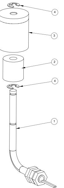
Figure 1-42 Float Switch w/ Polypropylene Barrel Assembly C-6549 Rev -
