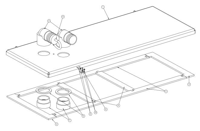
70 Gallon Universal Recovery Tank Cover Assembly Parts List
