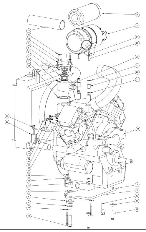
Figure 1-13 Engine Assembly - Front View D-5572 Rev G
