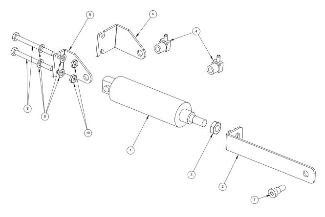
**Diverter Valve Actuator Assembly Parts List**
